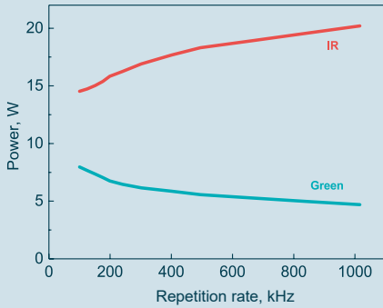
Average power dependence on the pulse repetition rate for infrared and green (SH option) output
