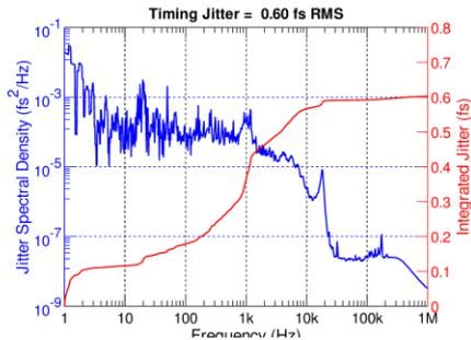
Out-of-loop timing jitter between two stabilized fiber link<sup>1</sup> above 1 Hz
