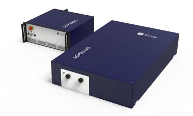
This femtosecond laser by Cycle is an ideal light source for various tasks in micro-machining, materials analysis and processing, semiconductor testing and more. With a center wavelength of 1550 nm or 775 nm and pulse durations below 350 fs, many applications can benefit from this state-of-the art ultrafast laser.
