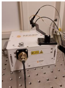
Photo of ALCOR 920-Mini2P coupled to a miniscope (taken by the “Mini2P team” at NTNU, Kavli Institute).
